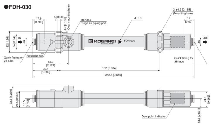
Note: Attach the piping so that the air flows in the direction shown by the flow direction mark. Sending the flow in the reverse direction will result in deterioration of dehumidification performance.
