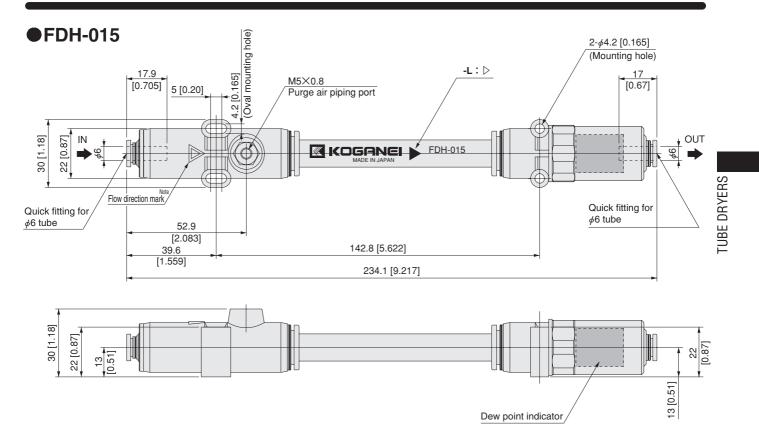
Note: Attach the piping so that the air flows in the direction shown by the flow direction mark. Sending the flow in the reverse direction will result in deterioration of dehumidification performance.
