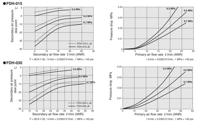
Conditions: Supplied air temperature at 25°C [77°F], water vapor in supplied air saturated at 25°C [77°F], purged air piping port open.
