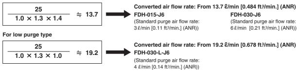
In this condition, the three models **FDH-015-J6**, **FDH-030-J6**, and **FDH-030-L-J6** are usable. Of these three models, we recommend use of **FDH-015-J6**, which has the smallest standard purge air flow rate.
