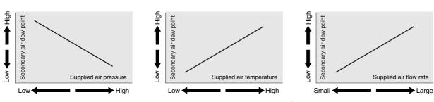
The air dryness increases with higher air pressure, lower temperature, and less flow rate for the supplied air.
