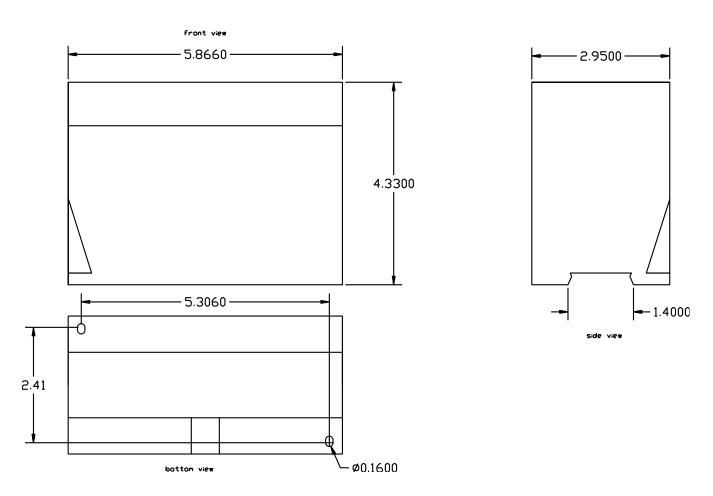
**Enclosure:** Gray polycarbonate with clear cover. Provides IP40, UL94V-1
