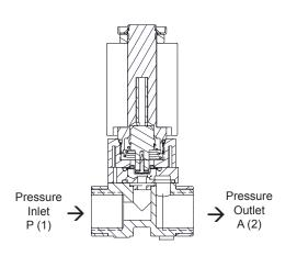
Position 1) Coil De-energized. Pressure inlet port P (1) is open to outlet port A (2).
