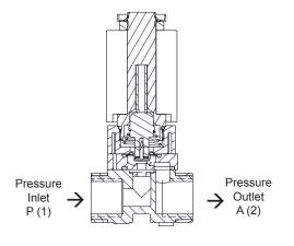
Coil De-energized. Pressure inlet port P (1) is open to outlet port A (2).
