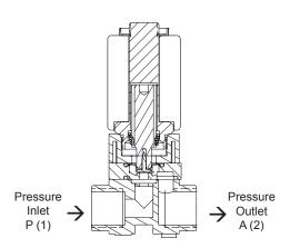
Coil De-energized. Position 1) Pressure inlet port P (1) is blocked to outlet port A (2).
