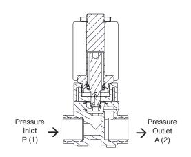
Position 1) Coil De-energized. Pressure inlet port P (1) is blocked to outlet port A (2).
