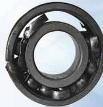
Catastrophic Cage Failure
