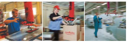
Our vacuum tube lifters are designed for lifts between 5 and 200 kg. They are simple to install, very easy to use and can be adapted to lift virtually any object.
