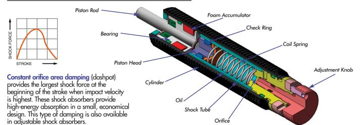
The damping force of an ITT Enidine single orifice shock absorber can be changed by turning the adjustment knob. Maximum damping force is achieved by turning the adjustment knob to eight (8), while minimum damping force is achieved by turning the adjustment knob to zero (0). Turning the adjustment knob causes the adjustment ball to increase or decrease the clearance (orifice area) between the ball and its seat, depending on rotation direction.
