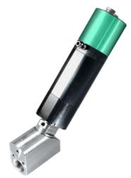
The FCV is available with 0-10 VDC differential or 4-20 mA differential command signal. Valve position monitor can be 0-10 VDC or 4-20 mA. Parabolic valve trim allows output to be linear and proportional to command input. Reduce trim of 3/4" available. The FCV contains a replaceable seat and trim.
