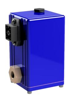
**PRESSURE RANGE** 0 to 150 psig (10 Bar) **ACCURACY | REPEATABILITY | ±0.5% F.S. | ±0.2% F.S.** MAX FLOW 0.8 SCFM (23 slpm) PORTS 1/8" NPT
