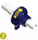
Twist the blue lock ring clockwise (approximately 75°) until audible "CPC Click" is heard. Alignment of the small blue lock ring rib indicator with the white body's rib indicator confirms final rotation is complete. 3 Snap the membrane pull tabs together and pull from connector.
