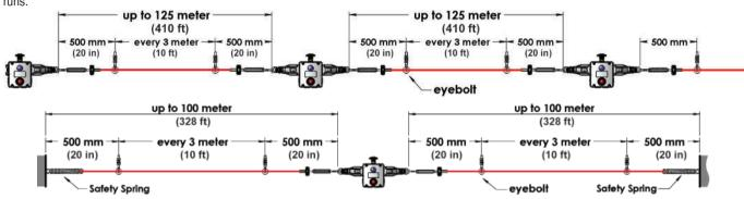
It is important that the first 500mm is not used as part of the active protection coverage. If protection is required in this first 500mm then it is recommended to use switches fitted with a mushroom type E-Stop button. IDEM also recommend when using a Safety Spring that a maximum of one corner pulley is used.
