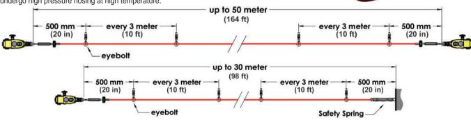
It is important that the first 500mm is not used as part of the active protection coverage. If protection is required in this first 500mm then it is recommended to use switches fitted with a mushroom type E-Stop button. IDEM also recommend when using a Safety Spring that a maximum of one corner pulley is used.
