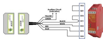
One switch connected to an SCR-2 or SCR-3 to give Dual Channel guard monitoring but with Automatic Start.
