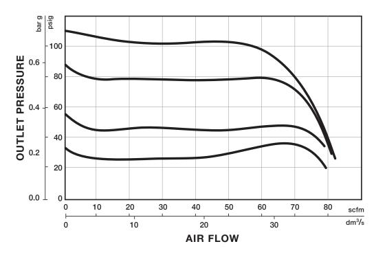
Inlet pressure: 145 psi (10 bar) Range: 4 to 145 psi (0.3 to 10 bar)
