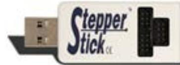
The StepperStick connects to the stepper motor mounted on the MPPV and can then be plugged into the USB port of a computer. This connectivity provides control through the device's digital interface. Since the computer can supply the power necessary for both the controller and the stepper motor, there is no need for an external power supply to drive the valve specifications.
