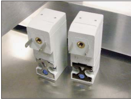
Position indicators- Silver plate indicates normally closed valve Black plate indicates normally open valve
