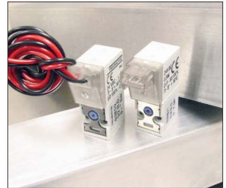
Position Indicators- Silver plate indicates Normally Closed valve, Black plate indicates Normally Open valve
