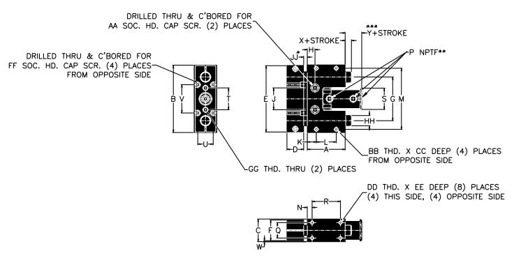
\*Dimension "JJ" (tool block extension - distance between the tool block and the body) is normally "0". On powered slides with internal cushions (Option "HC"), dimension "JJ" is 1/8". To order Special Dimension "JJ", see page 7 for special options and page 8 for ordering instructions.
