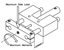
USE TABLE #4 TO CALCULATE THE WEIGHT THAT CAN BE CARRIED BY A PARTICULAR POWERED SLIDE (GIVEN BORE AND STROKE) THAT WOULD NOT DEFLECT MORE THAN A GIVEN AMOUNT. FOR EXAMPLE: WHAT WEIGHT CAN BE CARRIED BY A POWERED SLIDE (WITH A  $1^{1}/2^{"}$  BORE AND 18" STROKE) THAT WOULD NOT DEFLECT MORE THAN .005? SOLUTION: (SEE TABLE #4) X .005 = 4.54 LBS
